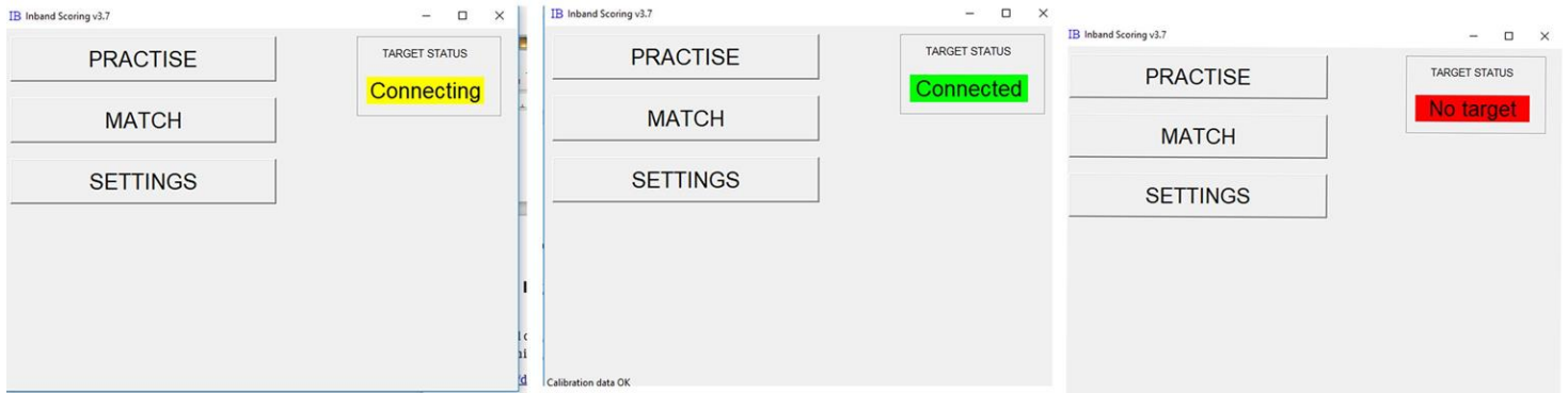
Picture 9. Executing InBand Scoring program. On the left picture, software is searching (yellow symbol “connecting”). In the middle, target is connected into computer and the system is ready to shoot (green symbol “Connected”. On the right, the target is not found (red symbol “No target”), and then you must check that the USB cable is connected, and the target power is on.
